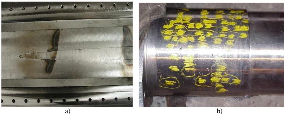
**Figure 2:** Defects observed: a) Steel Island on top, and b) Sands, opposite to the feeding side.
