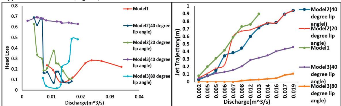
Fig. 2. (a) Energy loss between weir and bucket; (b) Jet trajectory
