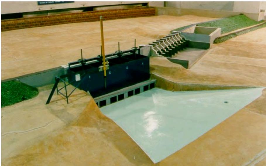
Figure 2. 3D Scale Model of the Porto Colombia Hydropower Plant
