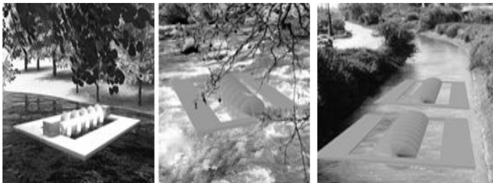
Figure 7: Photorealistic views of a schematic AWCT and two virtual representations of floating rotors in Evinos River and an irrigation channel.
