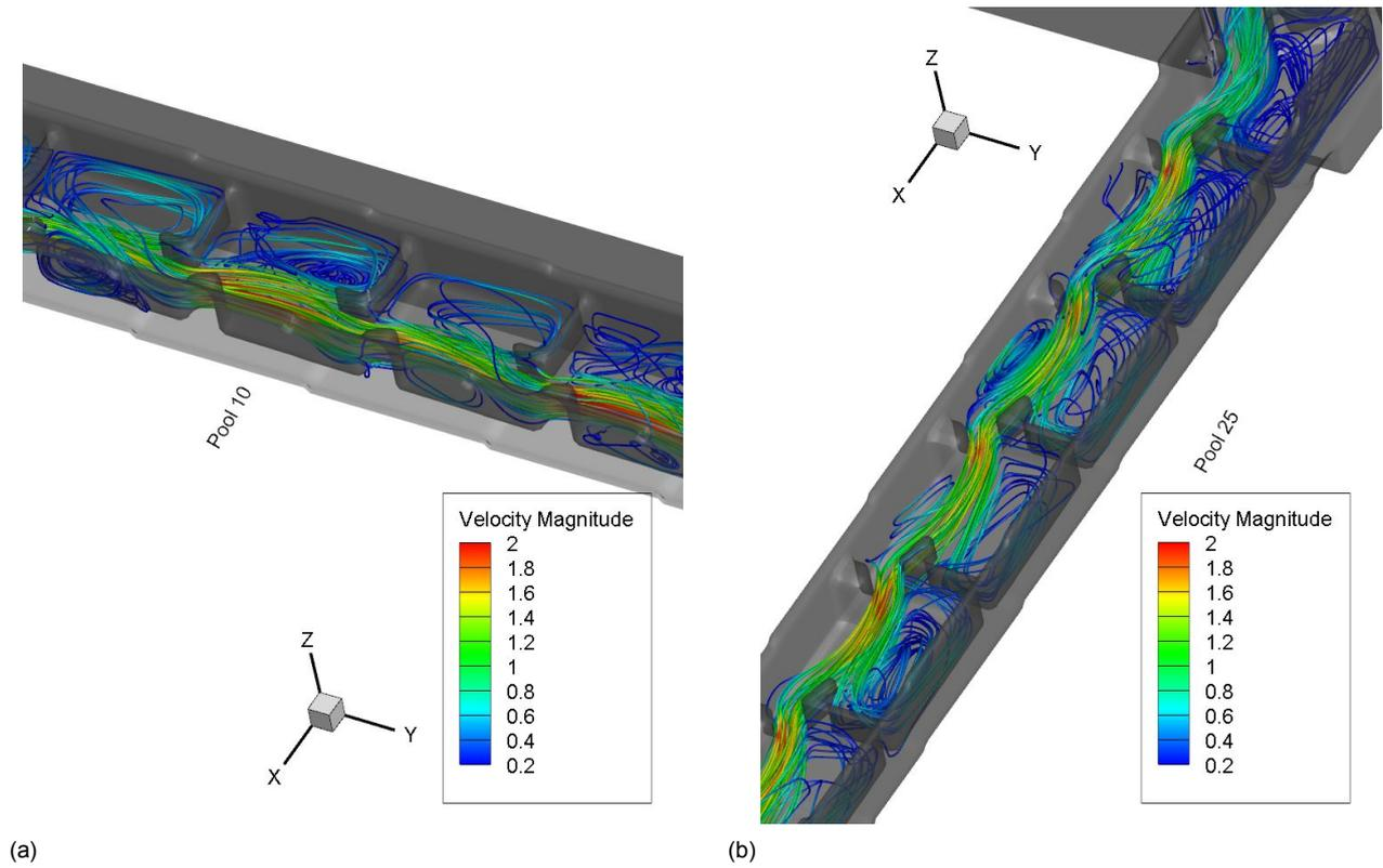
Figure 6 Simulation results of the vertical slot pass, 3D view, streamlines coloured by velocity magnitude;(a) first part,(b) after 2nd bend
