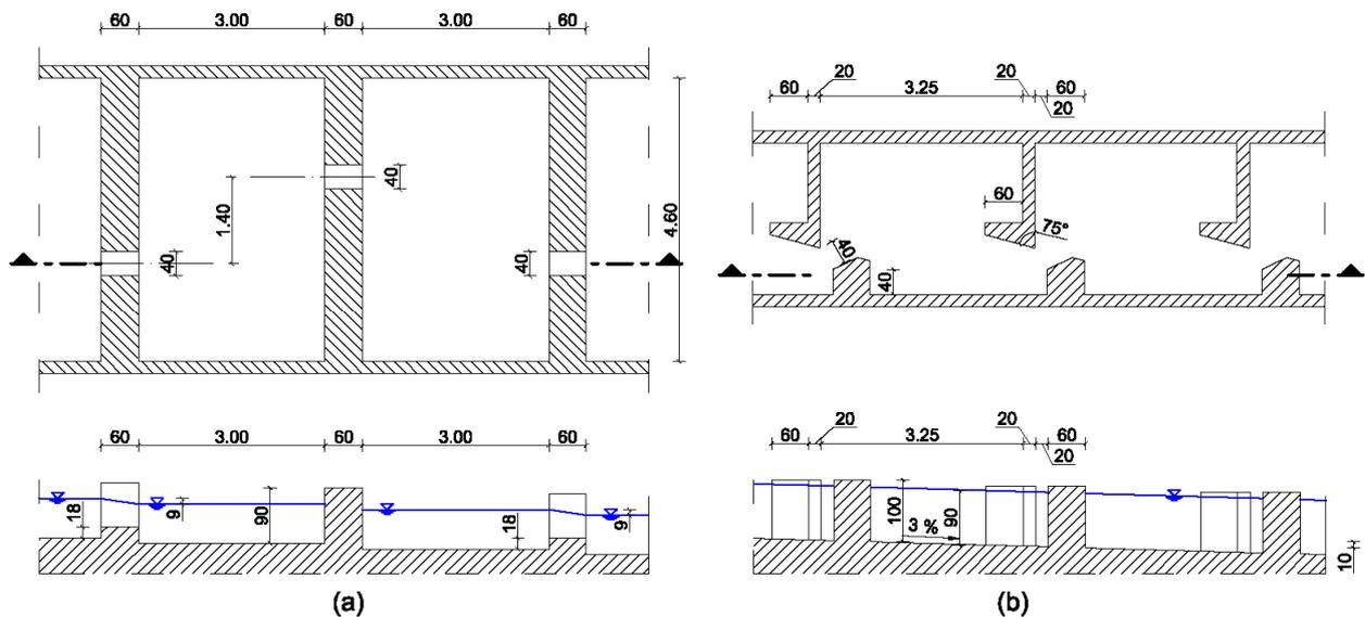
Figure 2. Geometry of designed fish passes, (a) crossbar block ramp, (b) vertical slot pass
