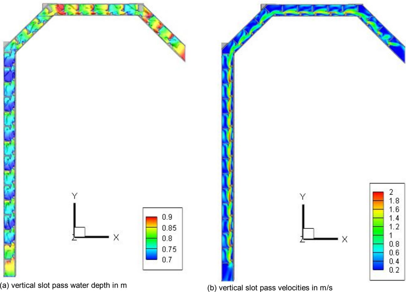
Figure 7. Simulation results of the vertical slot pass, plan view, (a) water depth in m, (b) velocities in m/s
