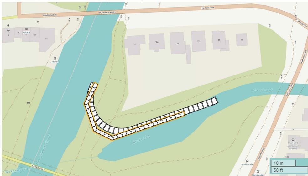
Figure 1. Location of the planned fish pass, black: crossbar block ramp, orange: vertical slot pass (map source: OpenStreetMaps)
