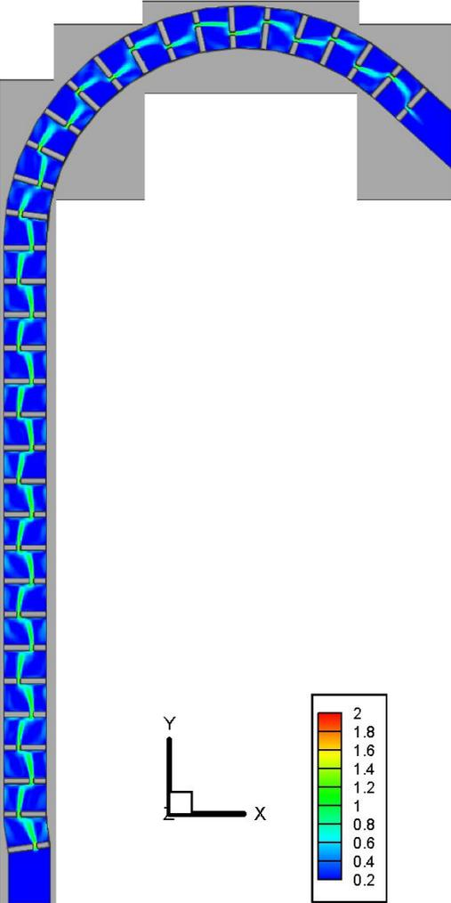
Figure 5. Simulation results for crossbar block ramp, plan view, flow velocities in m/s
