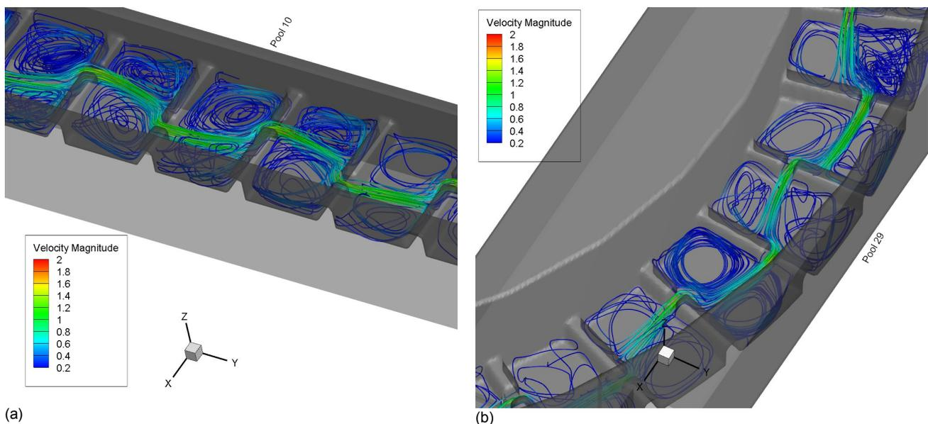
Figure 4. Simulation results for crossbar block ramp, 3D view, streamlines coloured by velocity magnitude;(a) straight part,(b) bend area
