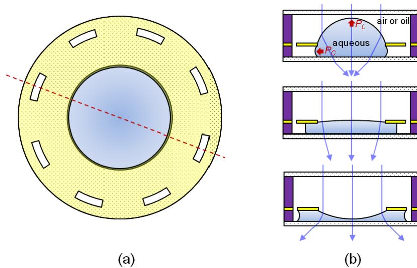
Figure 2. Schematics of the MEFL; (a) top and (b) cross-sectional views.
