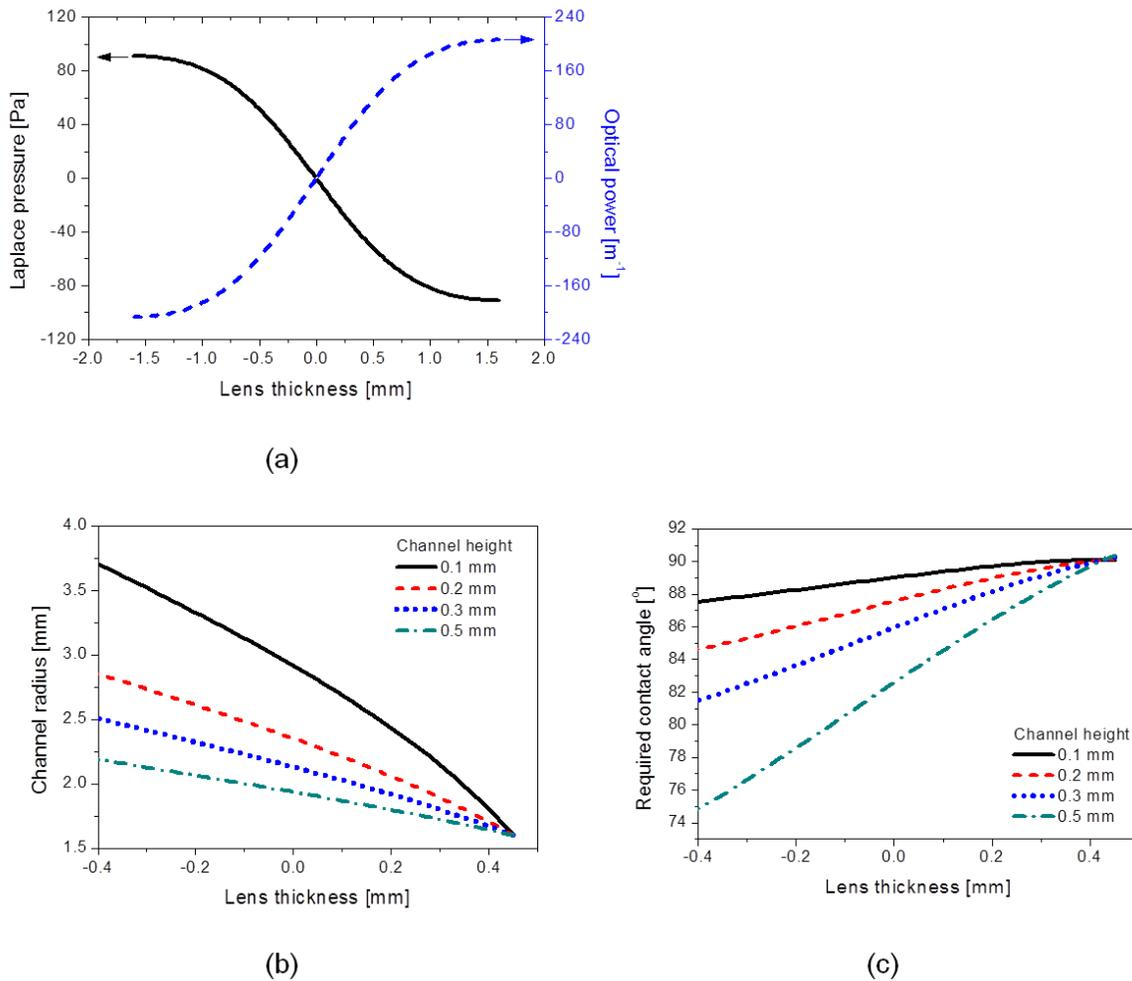
Figure 4. (a) Laplace pressure and optical power, (b) required channel radius, and (c) required contact angle according to the channel height depending on the lens thickness for the MEFL.
