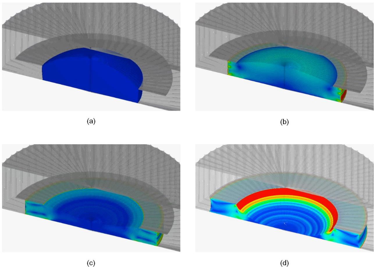
Figure 3. Flow-3D simulation results of the relationship between the channel radius and the lens height for the MEFL.
