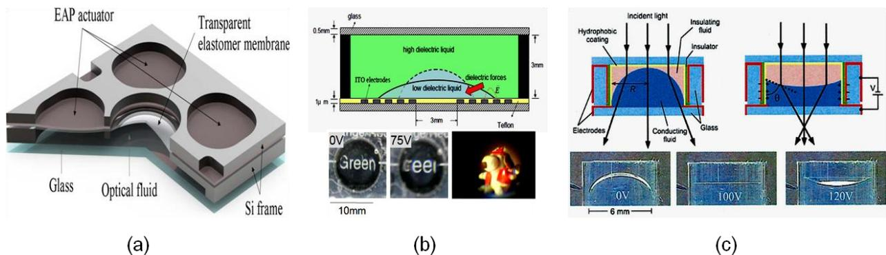
Figure 1. The previous tunable liquid lenses controlled by (a) electroactive polymer actuators [2], (b) dielectric force [3], and (c) electrowetting [4].
