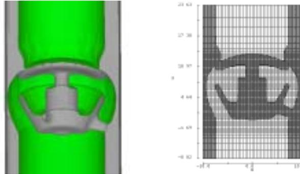
Fig. 1. Geometry and mesh about the valve piston. (a) Geometry at  $t=0$ , (b) mesh in  $x$ - $z$  plane ( $x$  and  $z$  in cm).
