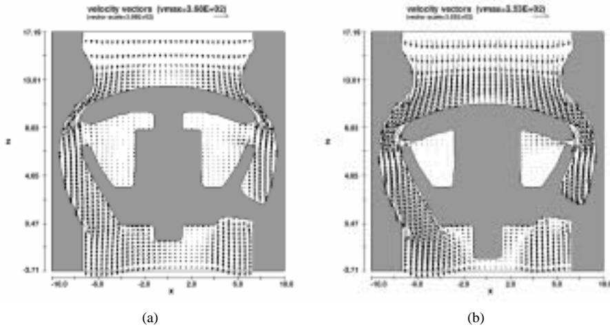
Fig. 2. Valve piston locations with pressure and velocity distributions at (a)  $t=0.6$  sec and (b)  $t=1.5$  sec.
