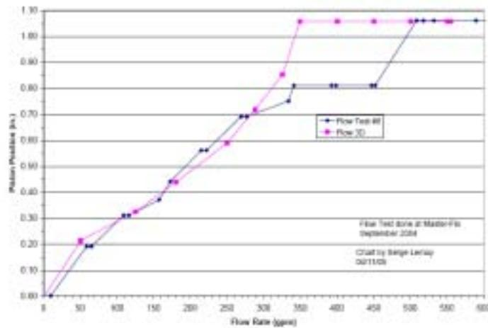
Fig. 3. Variation of piston position with flow rate (Courtesy of Stream-flo Industries Ltd)
