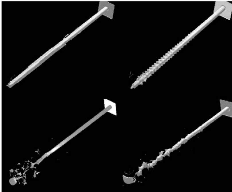
Figure 9. The shape of a fluid jet emerging from a round hole after it moves a distance equal to 25 lengths of its diameter. Top left - standard method, top right – semi-Lagrangian method, bottom left – standard method with surface tension, bottom right – standard method with surface tension.
