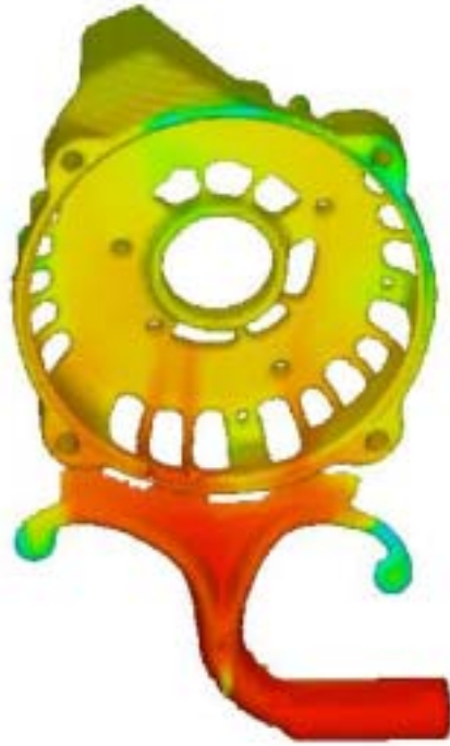
Figure 5a. NADCA part (left) at end of filling. Color indicates temperature.
