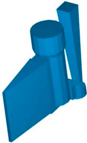
Figure 9. Wedge with riser and sprue. Chill plate is placed in sand mold at its thin end.
