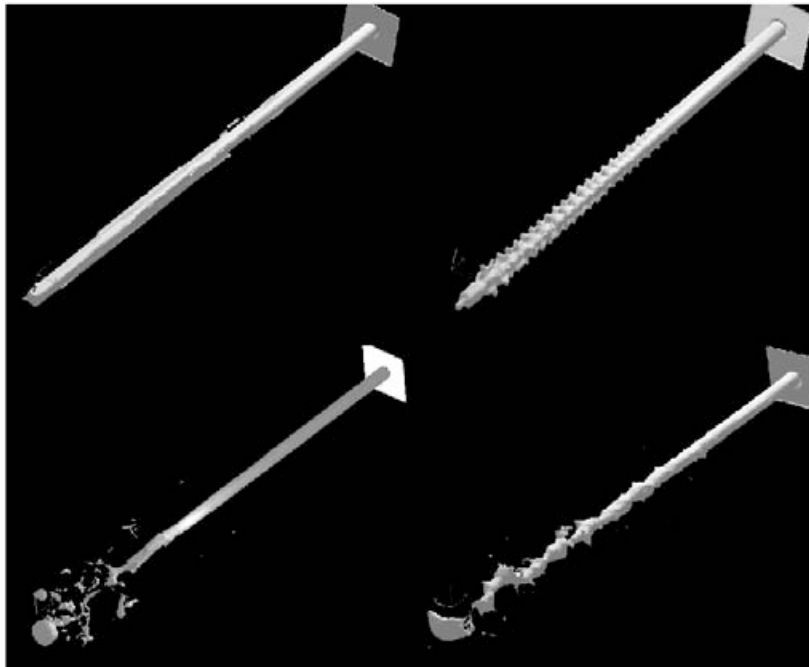
Figure 9. The shape of a fluid jet emerging from a round hole after it moves a distance equal to 25 lengths of its diameter. Top left - standard method, top right – Lagrangian method, bottom left – standard method with surface tension, bottom right – standard method with surface tension.
