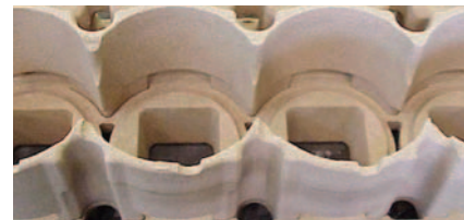
Core prints for casting with internal geometries must be sufficiently vented to avoid core gas blow defects.
