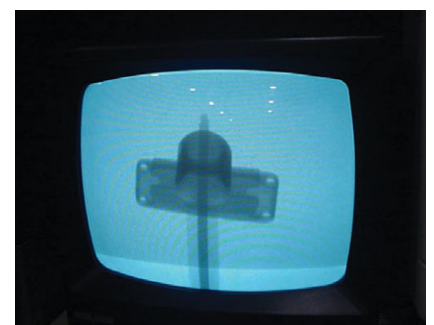
X-rays at different angles of a sample final part from the shop floor show no problems.
