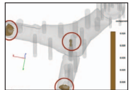
Defect locations due to incomplete drying. Courtesy of BMW.
